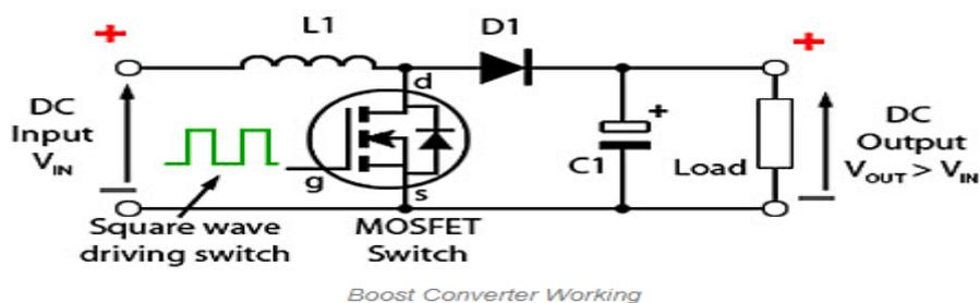
During the OFF period of second transistor the inductor L is charged and the capacitor C is discharged. The inductor L can produce the back e.m.f and the values are depending up on the rate of change of current of the second transistor switch. The amount of inductance the coil can occupy. Hence the back e.m.f can produce any different voltage through a wide range and determined by the design of the circuit. Hence the polarity of voltage across the inductor L has reversed now.
